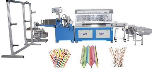
The machine RZM-500 is suitable for producing different size of paper straw such as 5 mm, 6 mm, 8 mm, 10 mm, 12 mm etc. with latest design for cutting device with 5 cutting knives. The stable working speed is 40-50 m/min.
